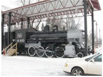
The Antigo "Consolidation" restoration was originally a UP engine saved for posterity. The 2-8-0 engine design either evolved from a 0-8-0 Pennsy (PRR) switch engine design with addition of a fixed front axle (by PRR shops) or it evolved from the popular 2-6-0 and thus a Baldwin design.
